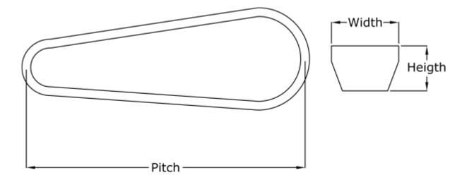
$\begin{array}{ll} \text{Datum Llength} = 1240 \\ \text{Height} &= 10 \\ \text{Length inside} &= 1220 \\ \text{Type} &= \text{BB46} \\ \text{Width} &= 17 \end{array}$
